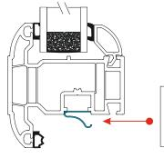
Fit a **BC001** Sash Spring to the sash on the center line of the stay fixing
